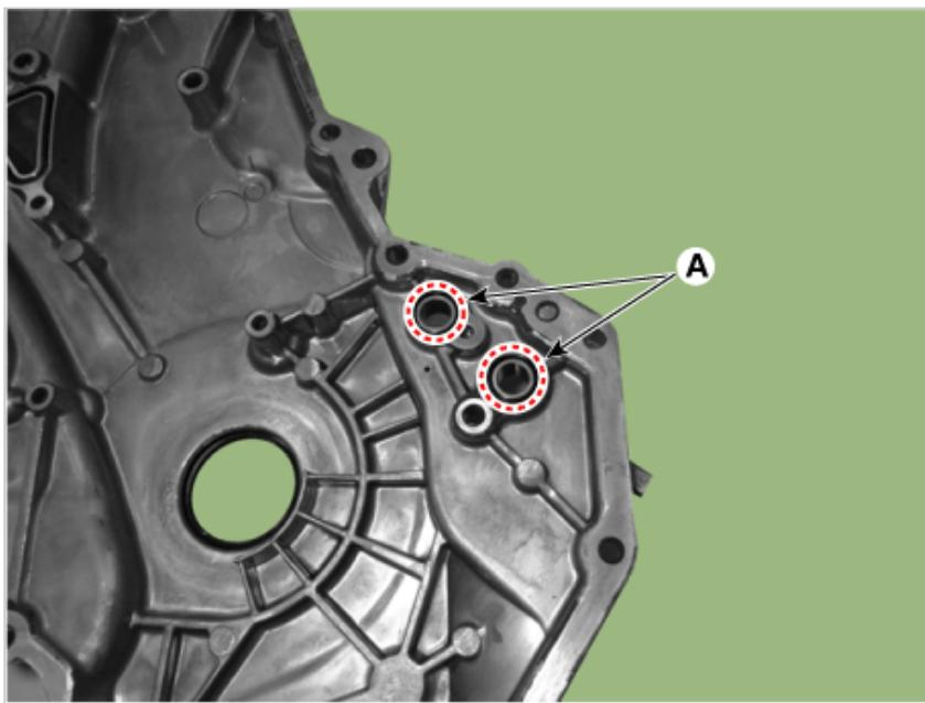
(3) Apply liquid sealant TB 1217H on timing chain cover. Assemble the part within 5 minutes of applying sealant.
