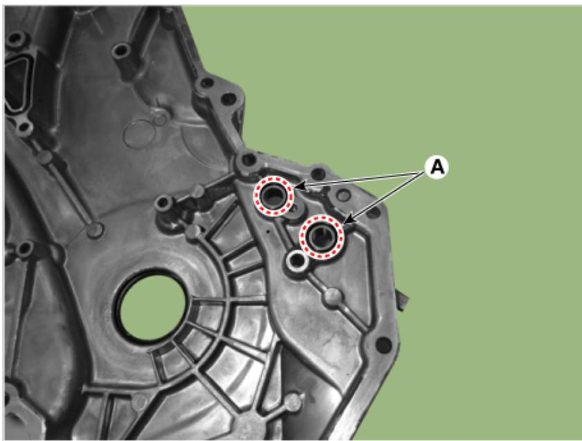
(3) Apply liquid sealant TB 1217H on timing chain cover. Assemble the part within 5 minutes of applying sealant.
